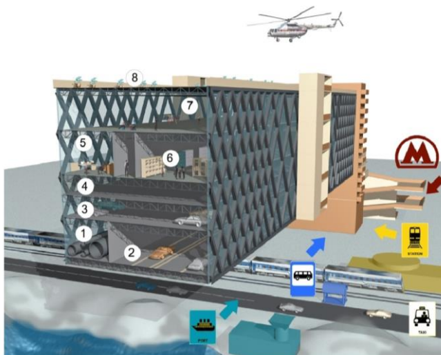
Figure 14. Cross-section of a bridge building with the functional contents of the floors: 1 – engineering communications transit, 2 – car passage, transportation links, 3 – buffer rooms: technical floor, parking lots, warehouses, etc, 5-7 – rooms of various functional purposes, 8 – operable roof (evacuation)
